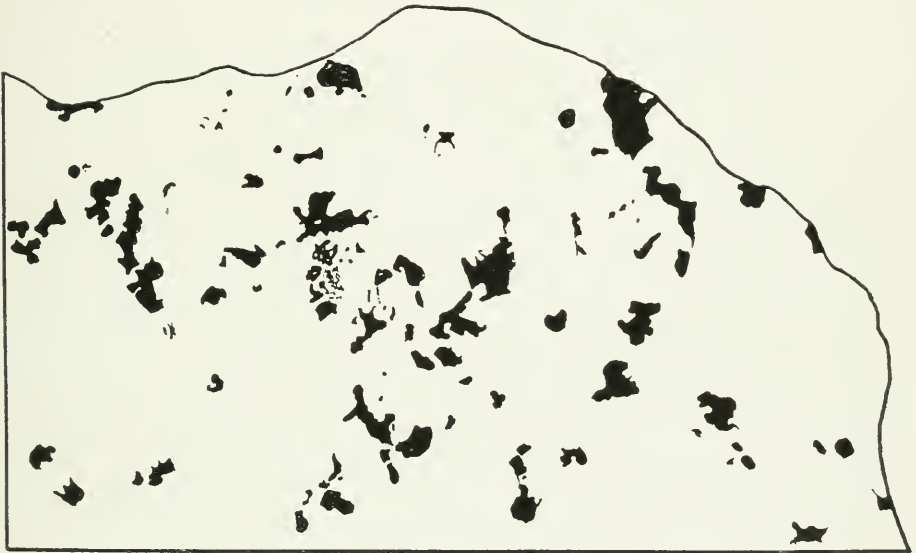
Fig. 26—"Spotted" granite, actual size. Black represents sulphides; white represents granite. The sulphides replace or impregnate the rock. Creighton mine, Sudbury area, Ontario.
